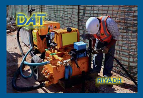
The construction of the tunnels and all the stations beneath the stratum level has required a geological study focused on soil permeability. The DAT instruments partnered consulting company is, in facts, the local member in charge of the test, undertaking double packer tests combined using DAT instruments Lugeon/
